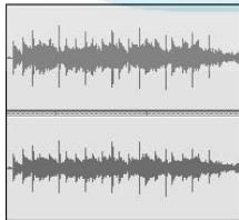
Figure 3-21: A stereo track (top) can be split into two mono tracks (bottom).
